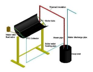
Fig: 2a. Schematic of Solar thermal Siphon Pump
