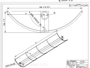
Fig: 3. Schematic of parabolic through collector.
