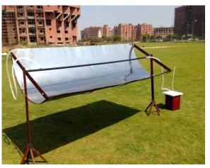
Fig: 2b. Working set up of solar thermal Siphon Pump at Sharda Univ Greater Noida campus
